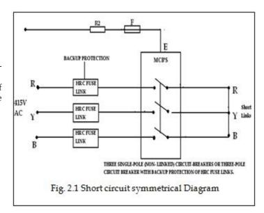
Mostly we can use MCCB / MCB's for protection purpose in electrical system. But we can't test the MCCB / MCB's before short circuit / over-loading it will work or not (Electromechanical devices)
